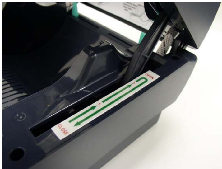
Fig. 1 Top cover support is fixed at position 2
